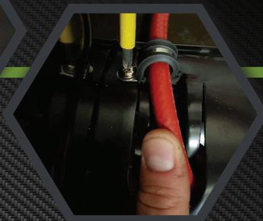
Now remove the 30amp fuse from the fuse holder to ensure the reel remains isolated while you carry out the remaining steps.
