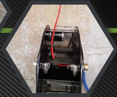
The 30amp fuse can now be placed back into the fuse holder and a final check carried out to ensure that the reel is free from any obstruction and is securely fixed in place.
